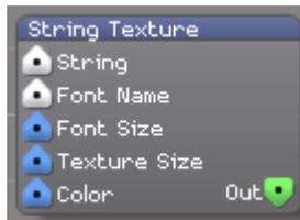
Uses the input string data to draw text with any font registered within the operating system.
