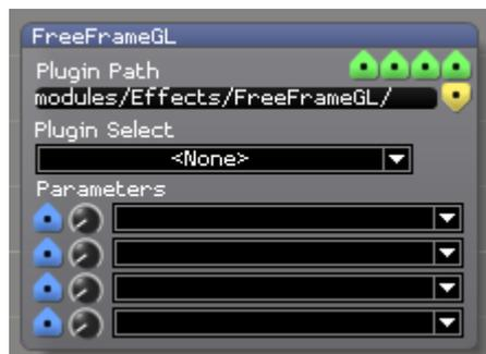
Processes the input texture using GPU powered FreeFrameGL effects and outputs the result as GLRender data. FreeframeGL video effects should be stored in the distrib/modules/effects/freeframeGL folder.
