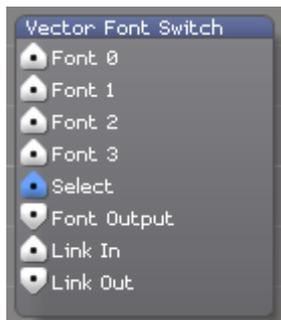
Outputs a specified Vector font based on the control value received at the select input.
