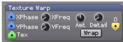
Deforms the texture received at the Texture input along the X and Y axis according to the frequency, amount and detail settings specified and outputs it to the GLRender stream .
