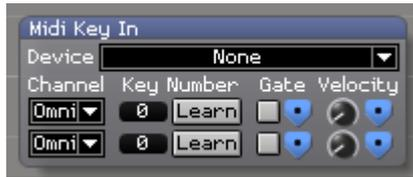
Specifies a Midi key input device and outputs the gate and velocity value.
