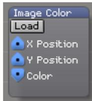
Outputs a vector containing a colour value based on the chosen X and Y location within a specified image.
