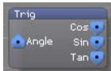
Outputs the cosine, sine, and tangent of the input angle.
