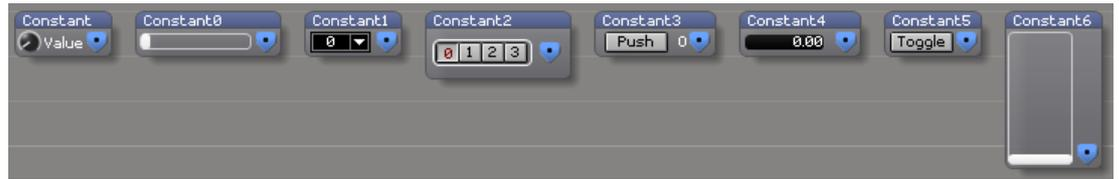
Outputs a user defined numeric value according to the value range and control type selected. The number value is stored internally as a 64-bit floating point number.
