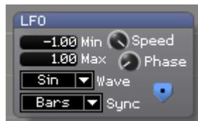
Outputs an oscillating control signal in the shape of a sin, saw, triangle, or square wave
