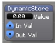
Stores the last value received at the input and passes it through to the output. When Ai quits out and restarts, the last value is recalled.
