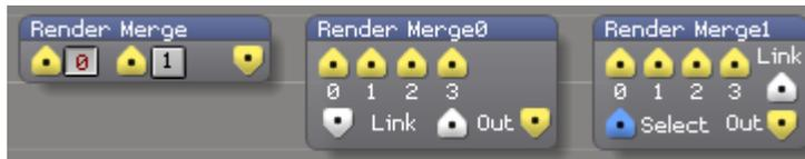
Renders each of the GL inputs in order, or renders a single specified input if the 'Select' input is connected.
