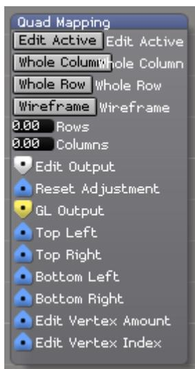
Allows for simple mapping of a video signal by adjusting the 4 corner points along the X and Y axis. This is similar to keystone correction but offers a greater amount of precision.
