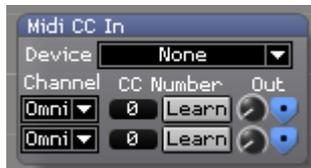
Outputs continuous controller ("CC") values received from an attached MIDI device
