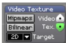
Streams video to the GPU and outputs a GPU texture containing the current video frame.
