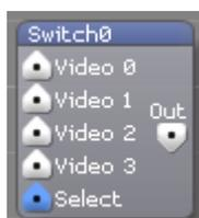
Outputs one of the input video signals based on the value of the 'Select' input
