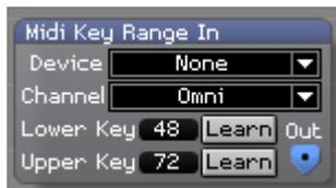
Specifies a Midi key input device, its upper and lower limit and then outputs the value.
