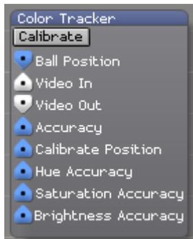
Allows for tracking based on colour for the signal received at the video input and then outputs the resulting information as control data.
