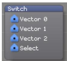
Selects one of the control signals and passes it through to the output
