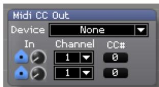
Sends continuous controller to an attached MIDI device ("CC") based on control values received at the inputs.
