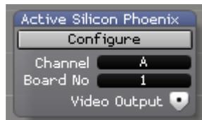
Allows for configuration of and output from an Active Silicon Phoenix HD SDI single or dual channel video input card.
