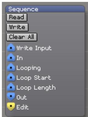
Captures a sequence of data from the input and replays it through the output according to the specified loop, start and stop options.
