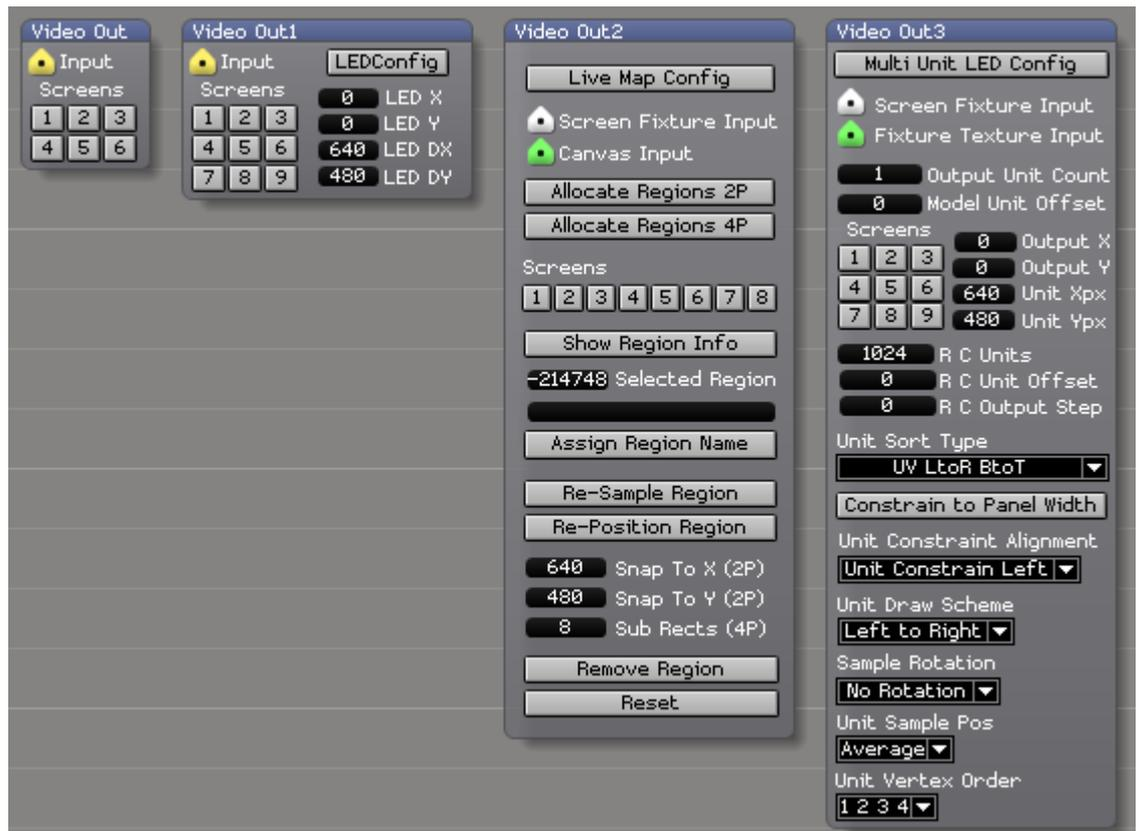
Takes the video input signal and allows the user to specify its output destination. Alternate skins allow access to LED config, Live Map and also to Multiple Unit Modular LED configuration options.
