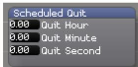
Automatically quits the AI system on the user specified hour, minute and second.
