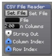
Allows a comma separated value file (CSV file) to be read according to user specified column and rows and outputs the value.
