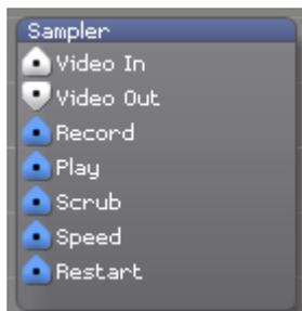
Samples, stores and replays a video signal received at the input.
