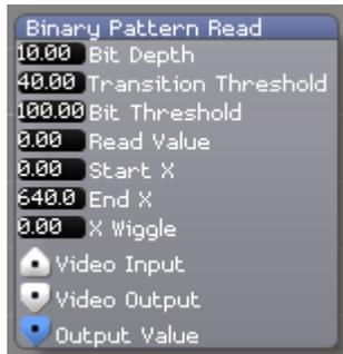
Module for interpreting data presented by Binary Patterns to the video input and outputting the resulting value as control data.
