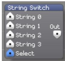
Outputs one of the input strings based on the value of the 'Select' input.
