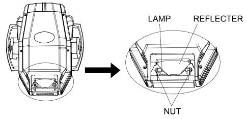
Lock the yoke before fitting/replacing the lamp.
