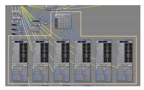
This part is pretty much straight-forward: each one of the six screens which are standing in mediaspinners on the ground is represented by its own screen fixtures so that each one can be loaded its own model (again, distinct by the UV mapping), and can be controlled, as per the y roation, via Artnet from the Mediaspinner controller.
