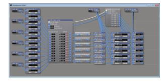
This subpatch simply allows to set the DMX addresses per mediaspinner - each one takes two DMX channels as 16bit. From the given start address per spinner, the next channel is computed. Then the ArtNet Input Large gets us the values, which are then being combined to a 16bit value (0...65,535), which is then normalized (0...1) and multiplied by the full travel (450 degrees). The result is returned, and used as y rotation parameter y Angle Adj. for the respective spinner.
