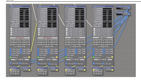
Finally, at the very bottom of the stagepatch, the projectors are defined. Note that again we didn't use softedge, but assigned each screen to a specific projector - see Advanced Output Patch for details.
