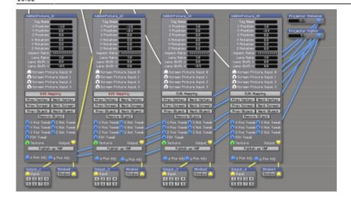
Finally, at the very bottom of the stagepatch, the projectors are defined. Note that again we didn't use softedge, but assigned each screen to a specific projector - see Advanced Output Patch for details (essentially it is dsabling Use All Fixtures per projector, and patching the screen fixture outputs to the respective inputs).
