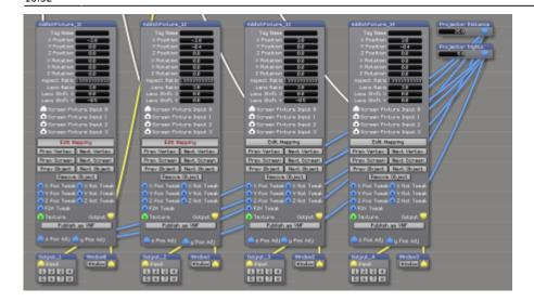
Finally, at the very bottom of the stagepatch, the projectors are defined. Note that again we didn't use softedge, but assigned each screen to a specific projector - see Advanced Output Patch for details (essentially it is disabling Use All Fixtures per projector, and patching the screen fixture outputs to the respective inputs).
