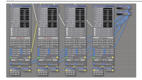
Finally, at the very bottom of the stagepatch, the projectors are defined. Note that again we didn't use softedge, but assigned each screen to a specific projector - see Advanced Output Patch for details (essentially it is disabling Use All Fixtures per projector, and patching the screen fixture outputs to the respective inputs).
