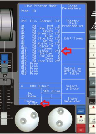
The fix is to make the personality with an 8 bit dimmer, and set the Dimmer fine channel to 0. Example here is the Elation Arena Par Zoom v2 15 DMX - you can use the
