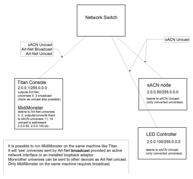
The question arose if the additional computer could be spared and if MIDIMonster could be run on the same machine Titan runs on. As explained in the section above this does **not** work with sACN - the external nodes see that MIDIMonster sends something but the values are always 0. I suspect this is due to some fancy network routing problem: two programs attempting to send on the same port and on the same machine, AND one program trying to listen to the other.
